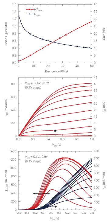
★ denotes the typical low noise bias point of  $V_{DS}$  = 0.5 V and  $I_{DS}$  = 80mA/mm (4 mA). The noise figure and gain plot is given for this bias and was obtained from on-wafer measurements. Data and models are available on request.
