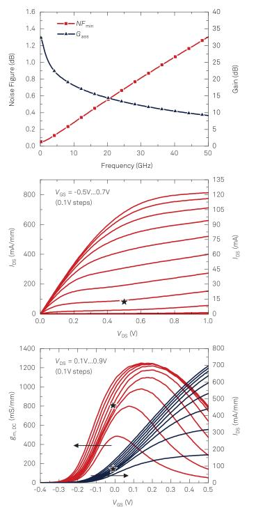
★ denotes the typical low noise bias point of  $V_{\rm DS}$ = 0.5 V and  $I_{\rm DS}$ = 80mA/mm (12mA). The noise figure and gain plot is given for this bias and was obtained from on-wafer measurements. Data and models are available on request.
