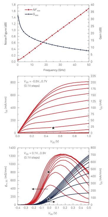
★ denotes the typical low noise bias point of  $V_{\rm DS}$ = 0.5 V and  $I_{\rm DS}$ = 80mA/mm (20 mA). The noise figure and gain plot is given for this bias and was obtained from on-wafer measurements. Data and models are available on request.
